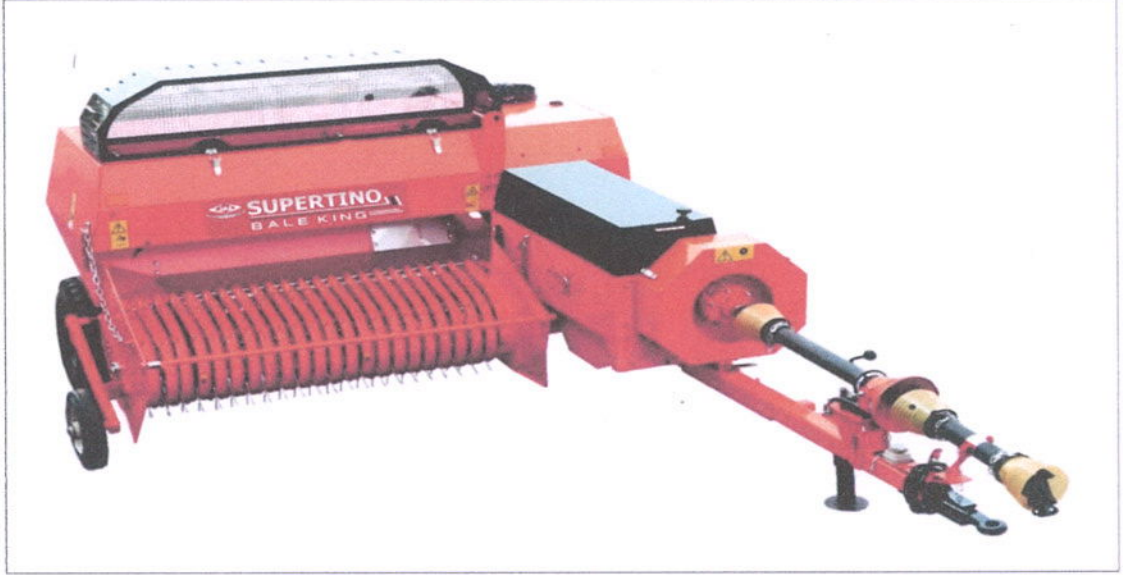
JAMNA, JAISB-165 SQUAR BALER (TRACTOR DRAWN, PTO POWERED)
